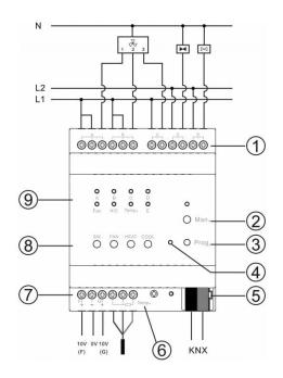
(1) 5 relay outputs: Configurable for fan speed (A/B/C), valve control (D for heating valve, E for cooling valve), or general switch output based on parameter settings.
